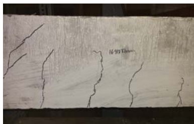
Fig. 3 Ductile Flexural (with steel fibres)
