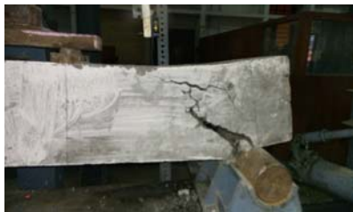
Fig. 2 Brittle shear failure (without steel fibres)
