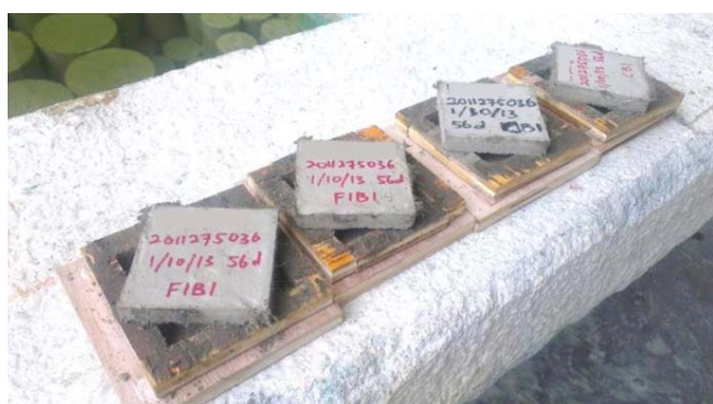
Fig. 2 Specimen used for Thermal Conductivity Testing
