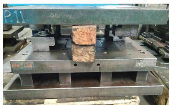
Fig. 5 QDC Housing (courtesy of PT.SPI)
