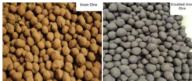
Fig. 6 Visual photos of iron ore pellets before and after steel dust coating
