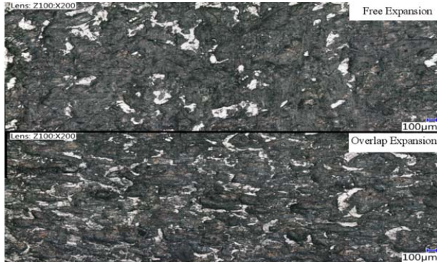
Fig. 12 Microscopic images for free expansion and overlap expansion with 11 mm host casing thickness
