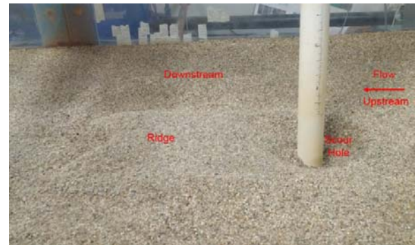
Fig. 4 Schematic of the scour hole and the ridge
