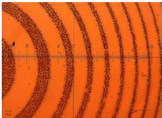
Fig. 4 Recorded Fresnel zone pattern on DDLC under polarized microscope
