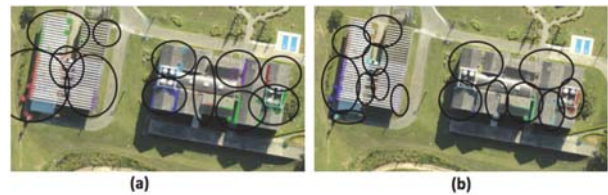
Fig. 7 Landmark Selection for the Aerial Mosaic using ORB. (a) is the Result for the X-Means in [22] and (b) is the result for the Proposed X-Means
