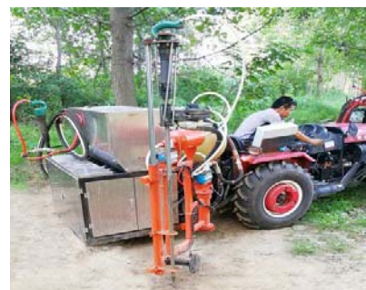
Fig. 5 Experimental prototype of orchard gas explosion subsoiling and fertilizer injection machine
