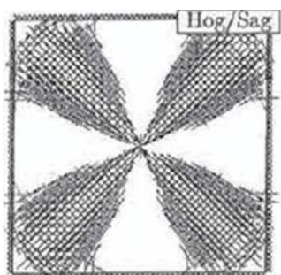
Fig. 5 Collapse Mechanism of a square clamped RC slab obtained with Jackson's lower bound solution [7]
