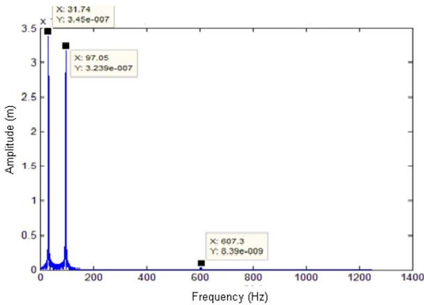
Fig. 4 FFT diagram of the intact beam using semi-analytical solution exposed to cosine force
