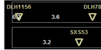
Fig. 16 Centerline Separation Range for two parallel runways with distances to preceding aircraft respectively touchdown
