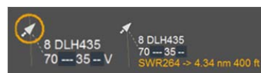
Fig. 14 Attention guidance elements for aircraft that have a short-term predicted conflict (orange circle around aircraft in automation level 0, orange alpha-numeric values in automation level 1)
