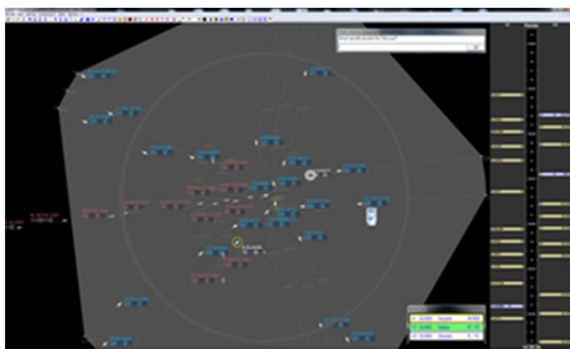
Fig. 10 DLR situation data display RadarVision with a radar screen on the left and a timeline on the right (overview of whole screen; more details in the following figures)
