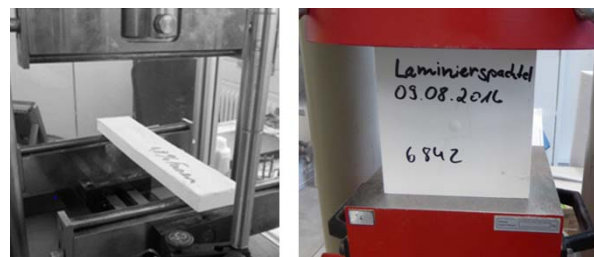
(a) Bending tensile strength (b) Compressive strength
