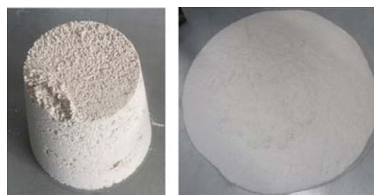
(a) Flow spread of mix 1 (b) Flow spread of mix 10
