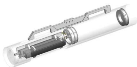
Fig. 3 Design of 2-MHz SSS Body
