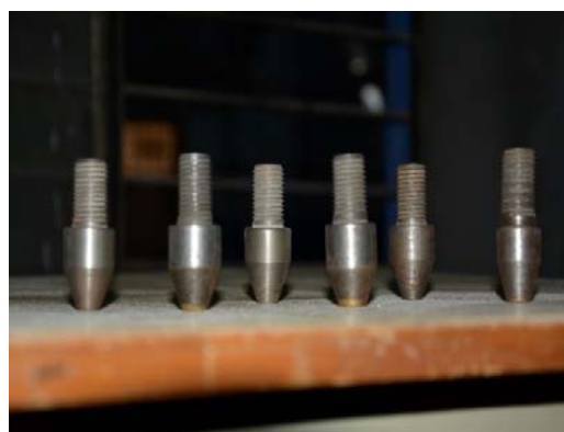
Fig. 8 Nozzles made of WC and HCHC steel
