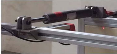
Fig. 3 Viscous fluid damper on STK
