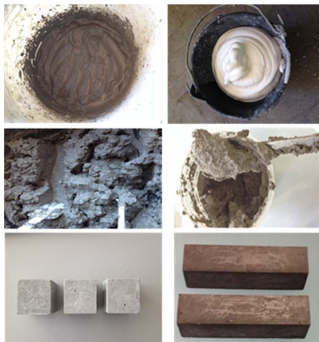
Fig. 1 Preparation of extrudable foamed concrete specimens
