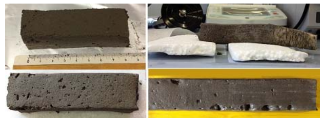
Fig. 2 Dimensional stability of extrudable foamed concrete at fresh state (green strength)
