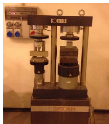
Fig. 4 Photograph of the test frame with twin columns used in the experimental campaign for the compressive and indirect tensile tests
