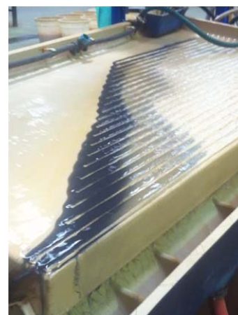
Fig. 7 Wilfley Table, High gravity ( 6^{\circ} ) stage of processing
