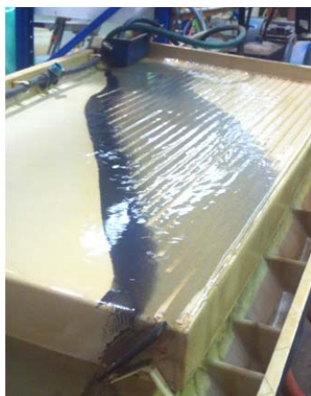
Fig. 6 Wilfley Table, low gravity stage ( 2^{\circ} ) of processing
