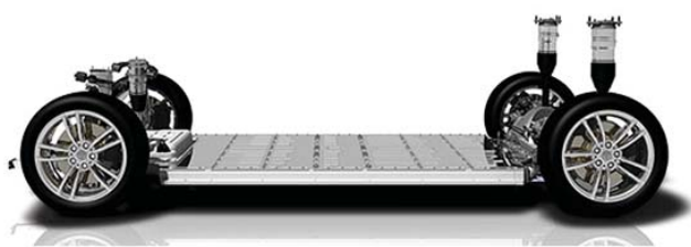
Fig. 4 Battery in a Tesla S Model chassis [24]
