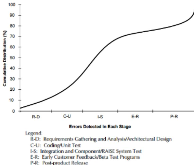
Fig. 1 Typical Cumulative Distribution of Error Detection [8]
