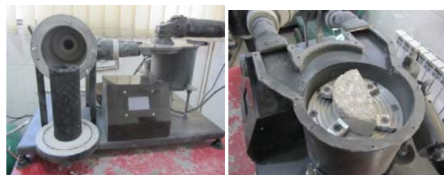
Fig. 11 The used devise to obtain concrete powder samples at different depth from the exposure surface [12]
