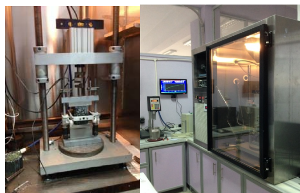
Fig. 3 Fatigue test equipment
