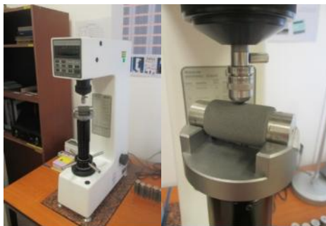
Fig. 4 Used Hardness Tester LECO LR-300TDL
