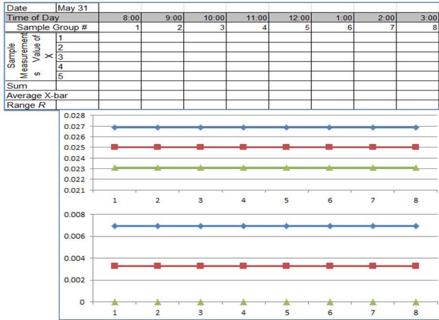
Fig. 5 Statistical process control chart for injection molding process
