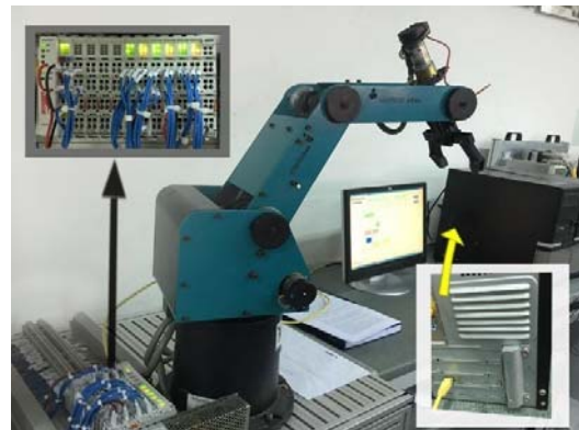
Fig. 7 Control system and robotics arm installation
