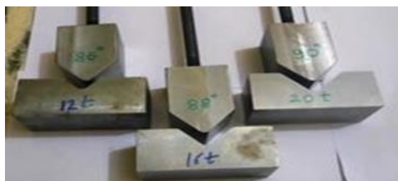
Fig. 2 (B) Punches and dies for experimentation
