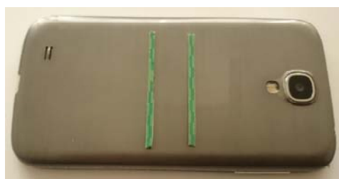
Fig. 14 2x2 MIMO antennas on the back, close to the center
