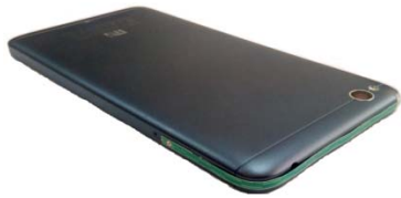
Fig. 9 Bending the new antenna to mount it on a small size mobile handset
