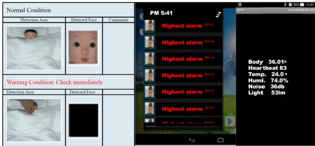
Fig. 5 Example of emergency alarm condition
