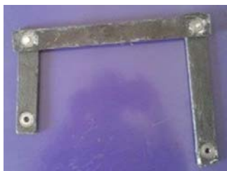
Fig. 6 Composite links of CR mechanism's prototype
