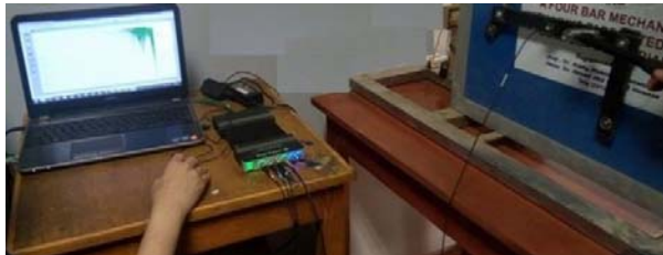
Fig. 7 Experimental test using dual channel analyzer
