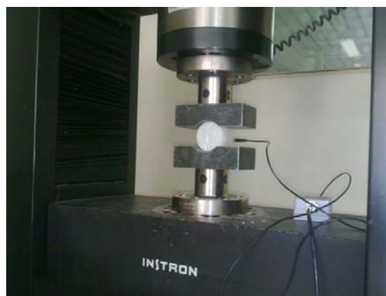
Fig. 2 Servo-electric loading frame with AE monitoring system
