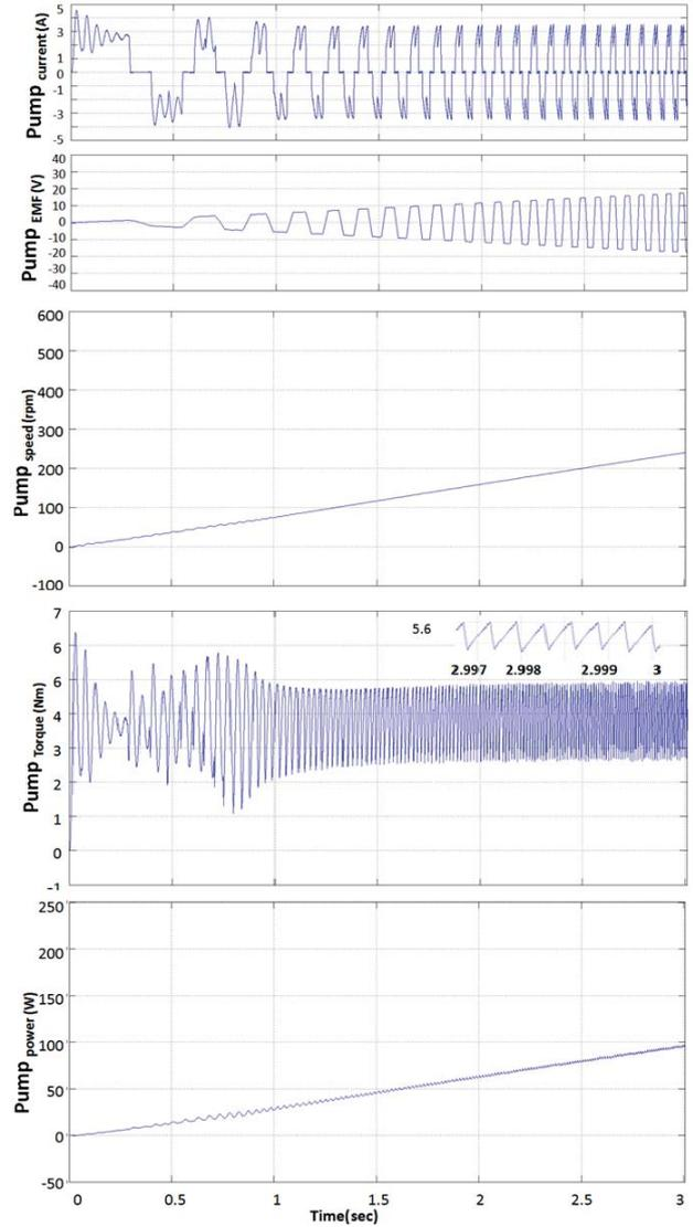
Fig. 11 BLDC-motor - water pump parameters at irradiance of  $600 \text{ W/m}^2$
