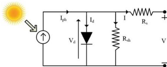
Fig. 2 PV Cell Equivalent Circuit
