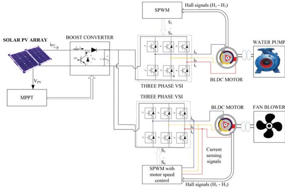
Fig. 1 Proposed SPV fed air cooling system
