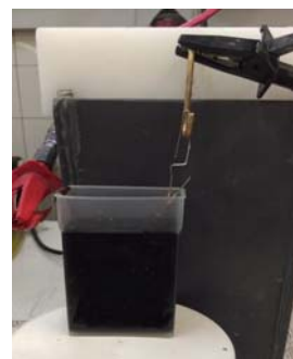
Fig. 1 The anodic EPD process of GO on Cu foil
