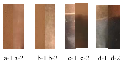
Fig. 2 Images of prepared samples after thermal annealing (a-1:0.01G-210, a-2:0.01G-510, b-1:0.01G-510, b-2:0.01G-520, c-1:0.2G-210, c-2:0.2G-220, d-1:0.2G-510, d-2:0.2G-520)
