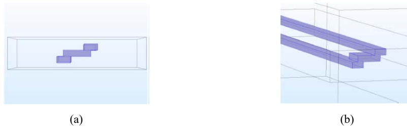
Fig. 5 Geometrical configuration of channels in design 3 from (a) front view (b) 3D view from the cantilever tip (c) maximum reflection for water, seawater, and milk (d) maximum deflection for blood
