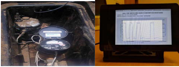
(c) Smart water meter (d) Raspberry pi with display Fig. 1 Real-time water-energy consumption data collection
