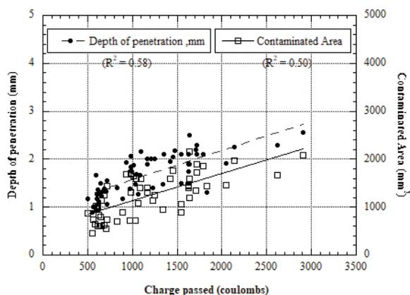
Fig. 8 Correlation between charges passed and depth of penetration and Surface area for concrete with crystalline waterproofing coating materials
