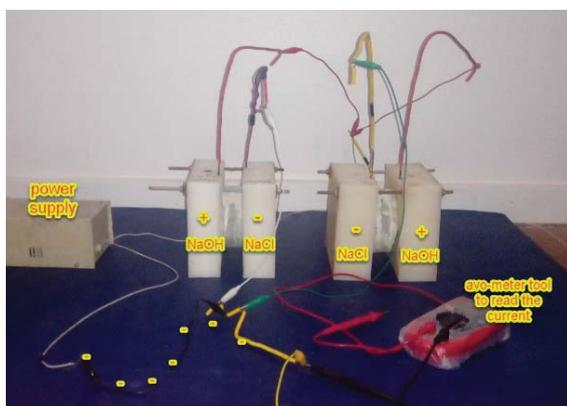
Fig. 2 RCPT setup
