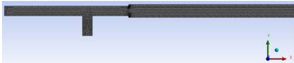
Fig. 2 Meshing of channel
