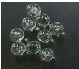
Fig. 1 (a) The spherically shaped of CRT glass as coarse aggregates used in this study
