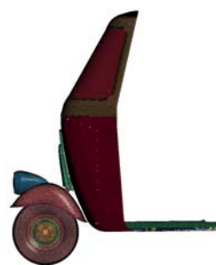
Fig. 1 FE Model of the front of the auto rickshaw
