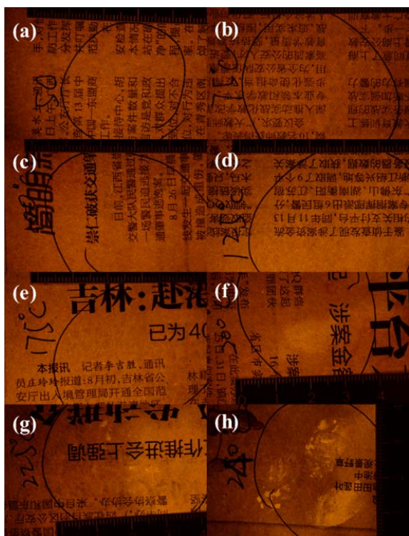
Fig. 3 The images of latent sweat fingerprints on newspaper under different temperature for 2 min (a) 50 °C (b) 75 °C (c) 100 °C (d) 125 °C (e) 175 °C (f) 200 °C (g) 225 °C (h) 240 °C
