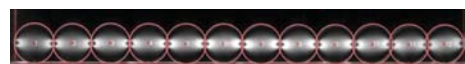
Fig. 18 One dimensional chain of photoelastic particles with marked circular boundaries of particles
