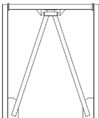
Fig. 1 The installation of the damper in frame
