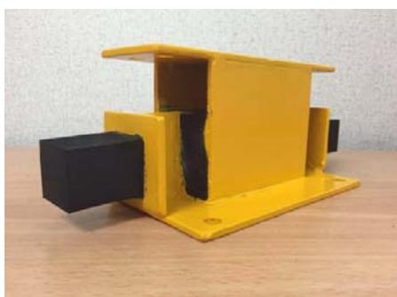
Fig. 2 The hybrid viscoelastic energy dissipation device
