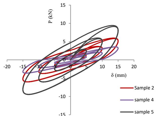
Fig. 7 (c) Cyclic behavior damper, effect of viscoelastic Shear area
