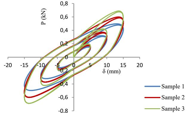
Fig. 7 (a) Cyclic behavior damper, effect of viscoelastic block volume
