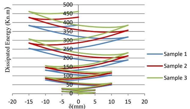
Fig. 7 (b) Cyclic behavior of damper, dissipated energy vs. Displacement
