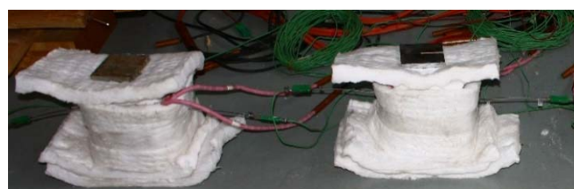
Fig. 2 HFRC specimens during the heat treatment
