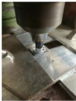
Fig. 5 Welding pin fixation in drilling holder
