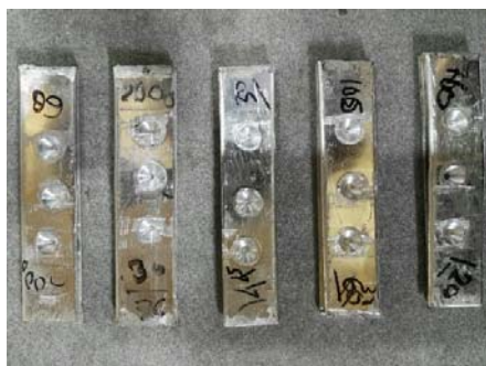
Fig. 11 Surface flash removal
