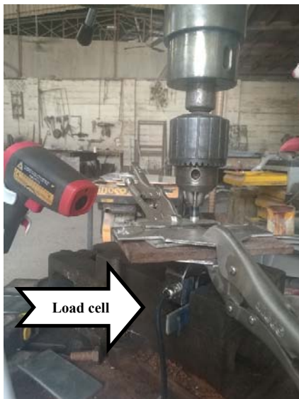
Fig. 6 Load cell and infrared temperature device arrangement
