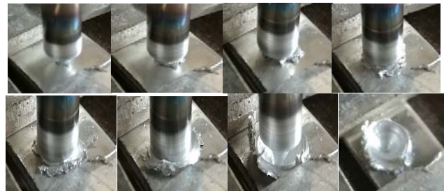
Fig. 8 Sequence of FSSW for AA1100
