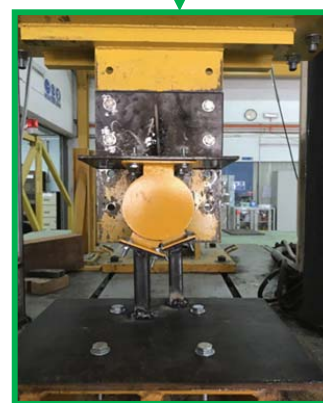
Fig. 2 The RRBD specimen in testing apparatus
