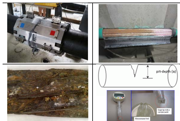
Fig. 1 Inspection procedure for corroded tendon
