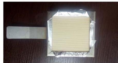
Fig. 2 Specimen and holder with final preparation
