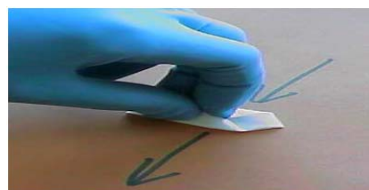
Fig. 3 Exemplification of how to hold the filter in order to clean the surface (based on [12])
