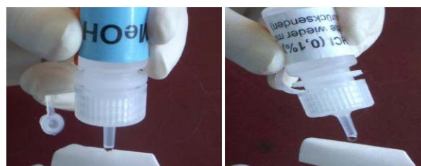
Fig. 2 Application of the fixatives (HCl and MeOH) to the paper filter (based on [12])
