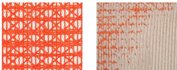
Fig. 2 The hybrid multi-axial seismic textile
