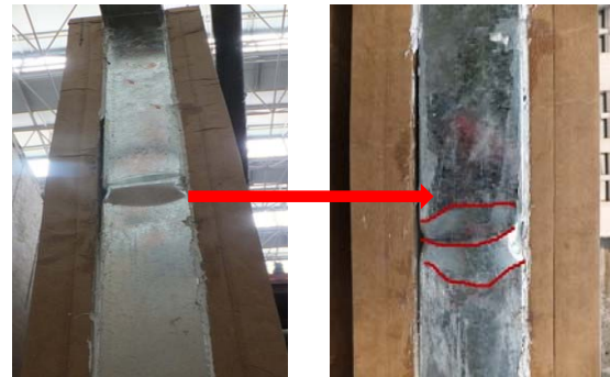
(b) Local buckling of W-2 CFS
