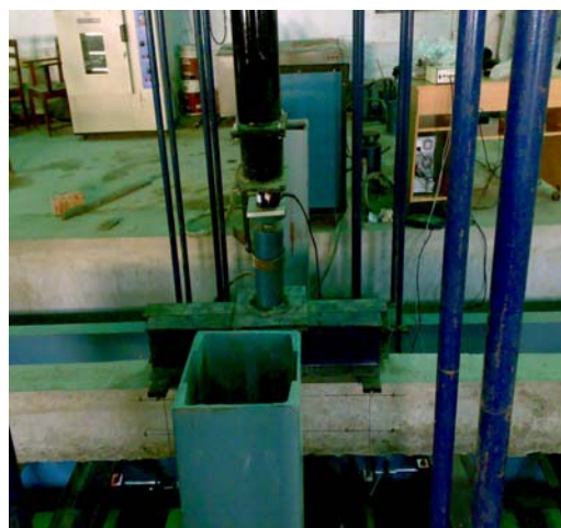
Fig. 7 Arrangement for flexural testing in Load Frame
